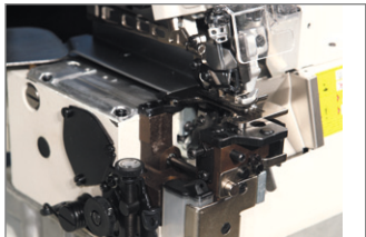
Optimized needle bar mechanism for noise and vibration prevention
