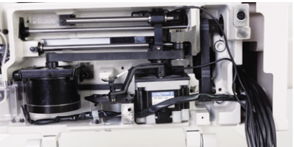
Independent operation of upper and lower thread trimmers
