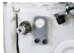
Upper Thread Detection System
