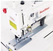
Thread tension adjustment by step motor
